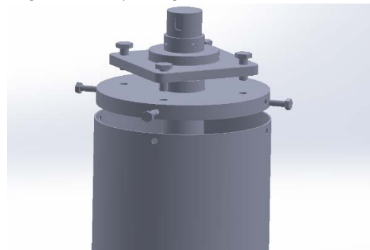
Fig. 14. Mounting the bearing and top plate on the shaft and the worm conveyor tube
