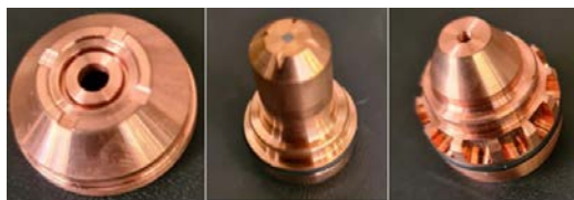
Fig. 18. New parts of plasma cutter torch for 200 A [4]
