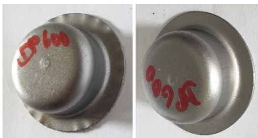
Fig. 1. Wrinkled and smooth flange cups after drawing with 4 kN and 7 kN blank holder forces respectively.
