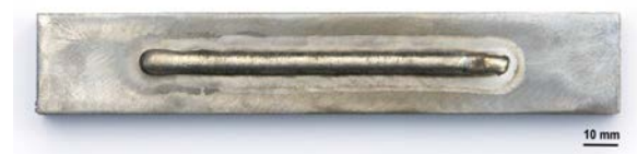
Fig. 8 Weld bead appearance CMT regime
