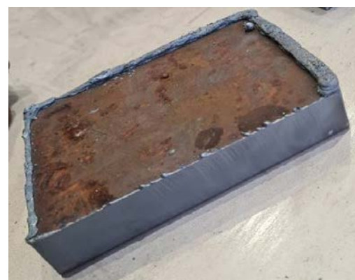
Fig. 21. Position of 25 mm with a lot of dross and oblique cut [4]
