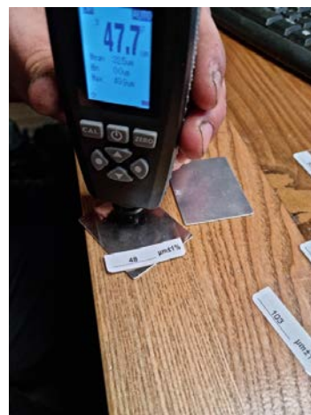
Fig. 14. Calibration of the device for measuring the thickness of the plasticized layer [5]
