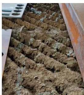
Fig. 11. Big amount of slag on the slat of the machine
