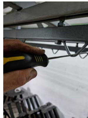
Fig. 7. Cleaning the suspension conveyor [5]
