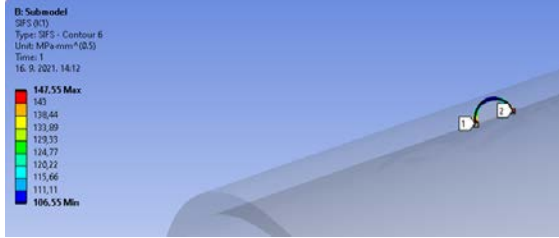
Fig. 4. Results of the numerical calculation of the crack stress factor, a=c=3.375 mm, p=5 MPa
