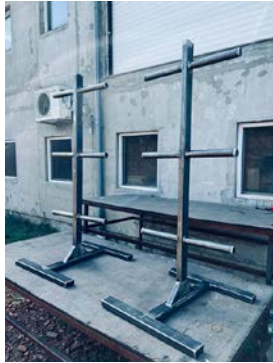
Fig. 8. Devices made of structural steel, without protection [5]
