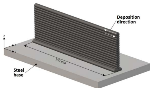
Fig. 1 Multilayer joint 3D model using the WAAM method
