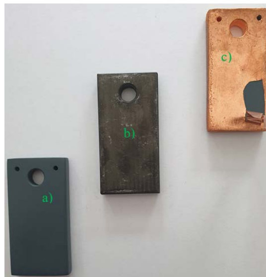
Fig. 10. Copper electroplating – electrically conductive primer
