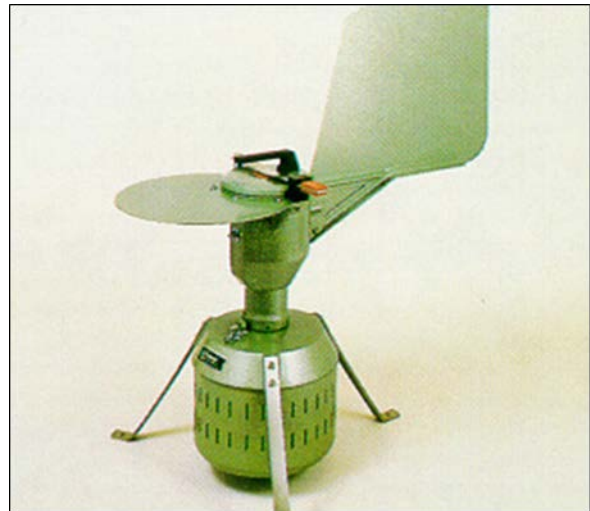
Fig. 3. Hirst-type (Burkard) pollen trap.
