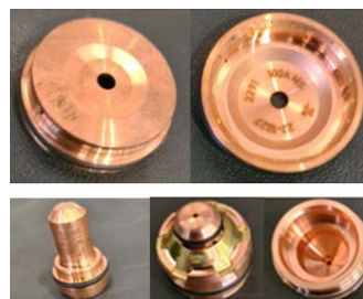
Fig. 13. New parts of plasma cutter torch for 100 A [4]
