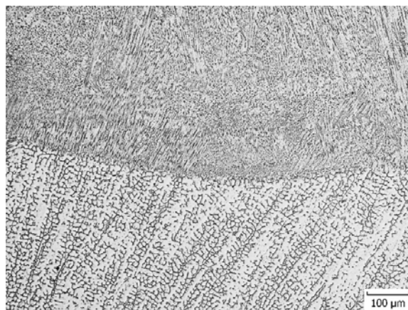
Fig. 2 Microstructure of weld metal - transition between layers
