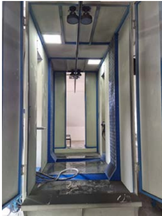
Fig. 3. Switched off powder collector [5]
