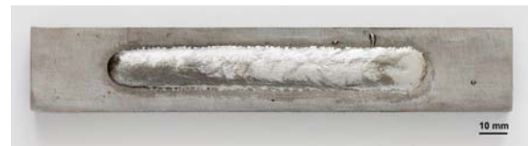
Fig. 7 Weld bead appearance of PMC regime
