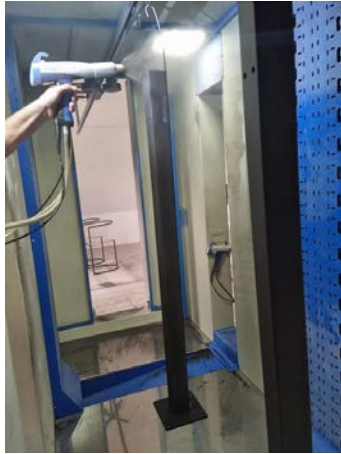
Fig. 11. Application with spray gun [5]
