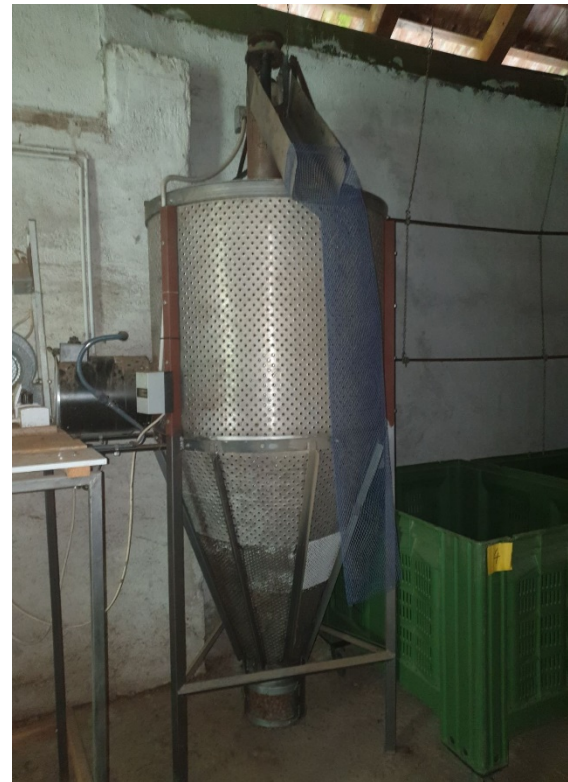
Fig. 5. A prototype of a dryer for hazelnuts was made
