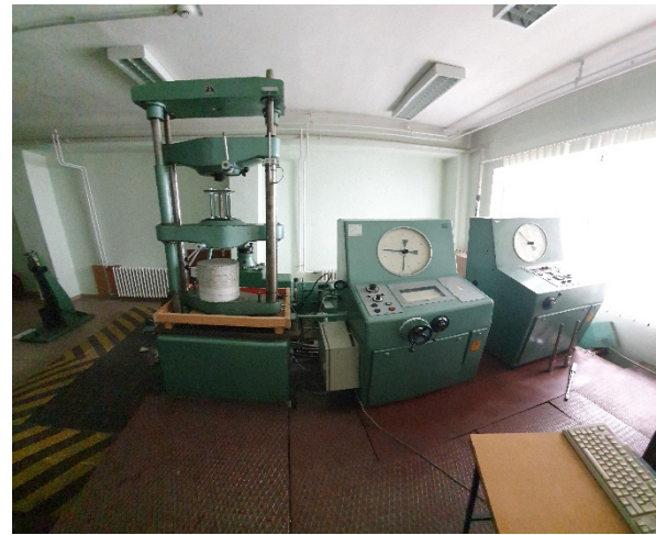
Fig. 2. ZD40 universal testing machine
