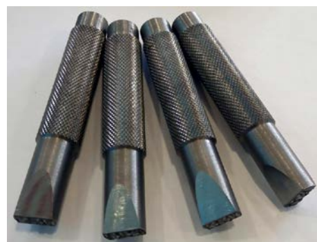
Figure 4. Stamps with rectangular marks after machining
