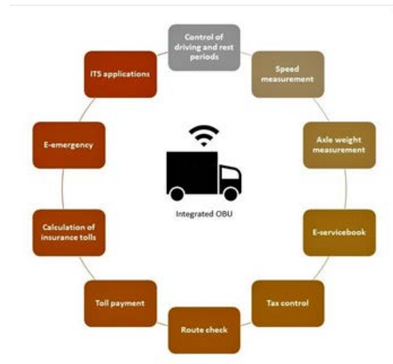
Fig. 1. Integrated OBU functions [Own editing]
