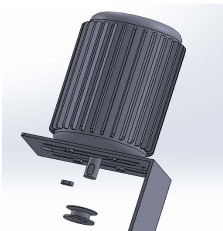
Fig. 11. Tightening the belt by moving the electric motor
