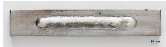
Fig. 6 Weld bead appearance of LSC regime
