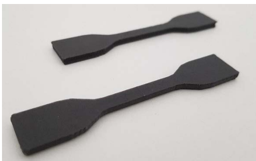
Fig. 4. Test bodies made on FDM device
