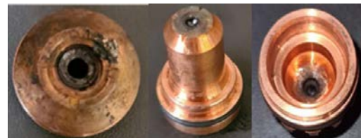
Fig. 20. Worn parts of plasma cutter torch for 200 A [4]
