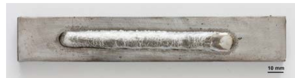
Fig. 5 Weld bead appearance of standard pulse
