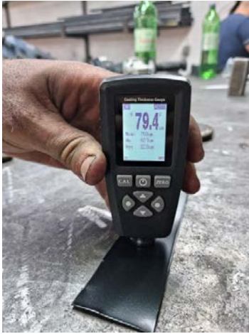
Fig. 15. Achieved thickness of plasticized layer [5]
