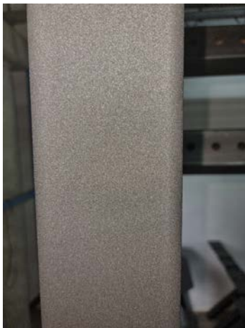
Fig 12. Texture and check of applied powder before baking [5]
